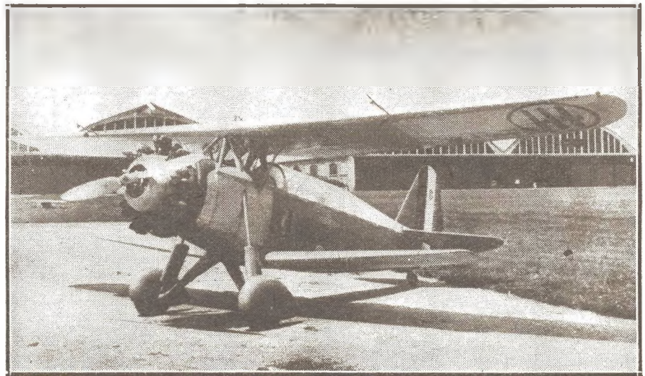
Classified as a trainer, the Jona J-6 seems advanced for that type work. Visibility from front pit, because of struts, is very poor.
