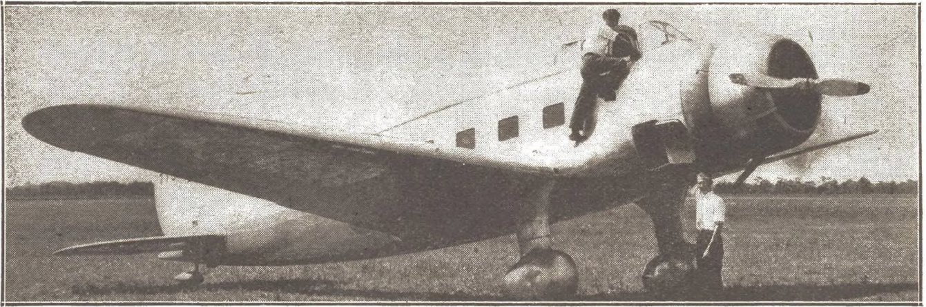
The General Aviation mail and express plane of 1934 was designed to carry a crew of one and six passengers. It used a Wright Cyclone engine of 710 h.p. and was of all-metal construction. Note fuselage baggage compartment and fixed landing gear legs.
