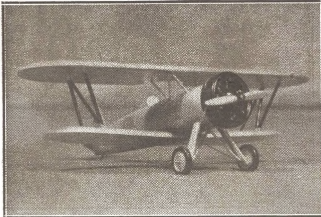
NAKAJIMA type 90 is used as a navy shipboard fighter. Looks like our 1932 Boeing P12-C. It is powered with a 450 h.p. engine.
