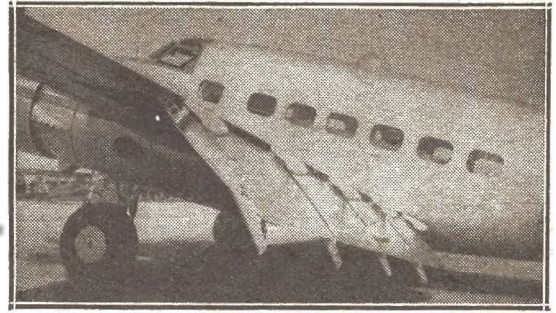
A close-up of the trailing edge camber-changing Fowler flaps at full extension on a Lockheed 14
